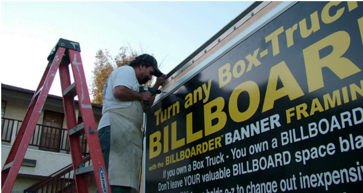
**Hook the capping plate over the base plate and screw the capping plate down onto the base plate utilizing the self tapping screws a foot apart and into and along the screw groove on the capping plate, which will tighten the banner further.**
