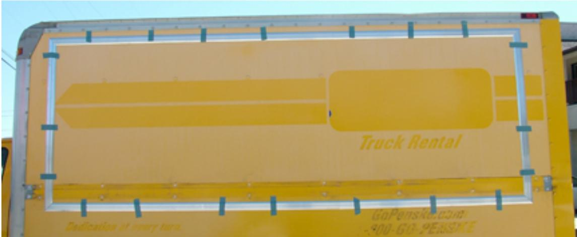
**Temporarily tape the four base plate sides into position using 6 inch duct tape holding tabs.** Tip: Start with the top side section(s) (that's the side with the pencil guide) then do the sides (keeping right angles to the top) and then the bottom. The temporary duct tape holding tabs make it easy to readjust and place all sections into the proper square 90-degree positions before screwing to the truck or wall. See photo above.
