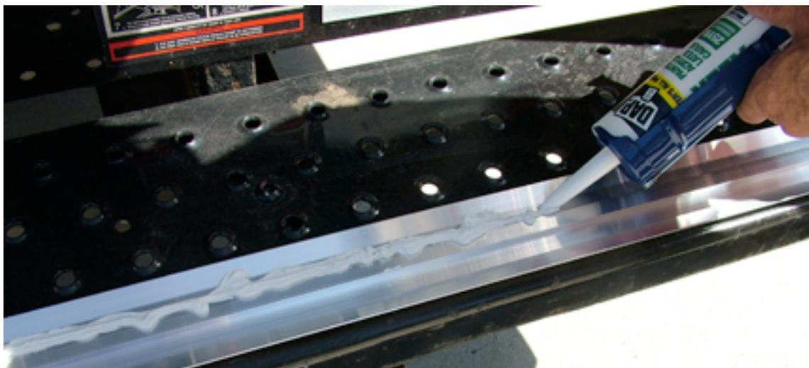
**Caulk the back of all the base plates to seal out air and water.**
